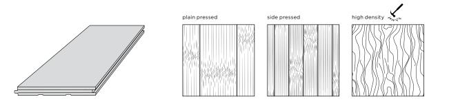
PP: Plain Pressed, SP: Side Pressed, HD: High Density, L: Lacquered Bona 80 gr/m<sup>2</sup>, LN: Lacquered Bona Naturale (extra matt) 125 gr/m<sup>2</sup>, O: Pre-oiled Woca Air Dried (has to be re-oiled after installation), SE: Sharp Edge, MB: Micro Bevel. \*) Middle layer cross pressed.
