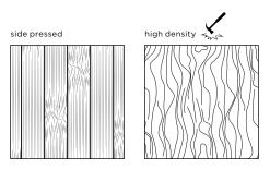
SP: Side Pressed, HD: High Density, L: Lacquered Treffert 80 gr/m<sup>2</sup>, BL: Brushed Lacquered 80 gr/m<sup>2</sup>, BSL: Brushed Stained-Lacquered Treffert 80 gr/m<sup>2</sup>, MB: Micro Bevel \*) Due to the characteristics of the high density bamboo, the 'depth' of the brushing will be different from one board to another. This creates a very natural effect.
