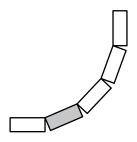
**flexible (F)** There are 2 different styles: solid strip (maximum width 17mm) and veneered strip (standard width 50mm).
