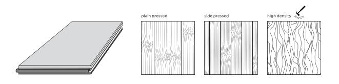
PP: Plain Pressed, SP: Side Pressed, HD: High Density, O: Pre-oiled Woca Air Dried (has to be re-oiled after installation), B: Bevel (only on length side)
